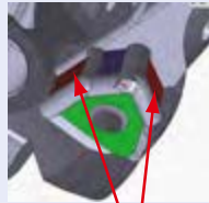
Inclined dovetail seat
